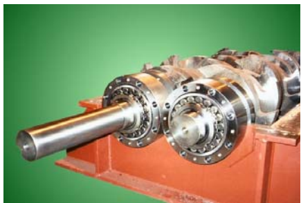
Picture 2: Counterrotating knives working mutually as backstop ( www.transdynamics.ca )
